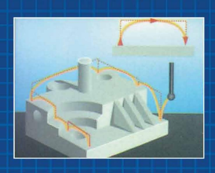
tower). "Continuous Motion Control" reduces cycle times by up to 30% by eliminating unnecessary machine moves and smoothing the probe trajectory.
