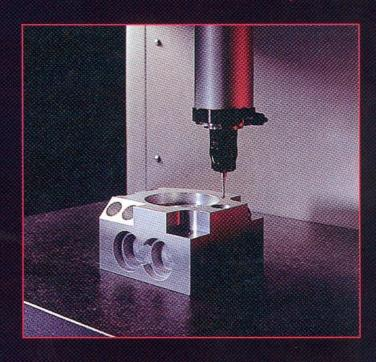
stroke. Component fixture design will further erode this critical dimension often forcing the selection of a larger machine. This adds to cost and reduces the CMM justification. With adjustable fixed pitch Z column (patent pending) Umpire ensures that regardless of probe, fixture design or application, the total Z measuring travel remains available and can be positioned exactly to suit specific needs.
